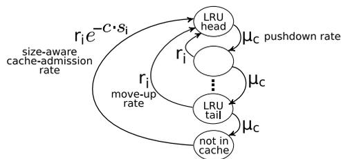
Figure 8: AdaptSize’s Markov chain model for object  $i$  represents  $i$ ’s position in the LRU list and the possibility that the object is out of the cache. Each object is represented by a separate Markov chain, but all Markov chains are connected by the common “pushdown” rate  $\mu_c$ . Solving these models yields the OHR as a function of  $c$ .
