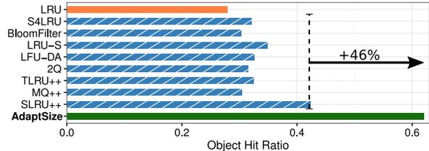
Figure 5: Comparison of AdaptSize to state-of-the-art research caching systems. Most of these use sophisticated admission and eviction policies that combine recency and frequency (striped blue bars). AdaptSize improves the OHR by 46% over the next best system. Policies annotated by “++” are actually optimistic, because we offline-tuned their parameters to the trace. These results are for the US trace and a HOC size 1.2 GiB.
