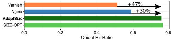
Figure 10: Comparison of AdaptSize’s implementation to the Varnish and Nginx production systems and SIZE-OPT. AdaptSize improves the OHR by 30-47% over the production systems and also achieves 99% of the OHR of SIZE-OPT. These results are for the HK trace; corresponding results for the US trace are shown in Figure 4.
