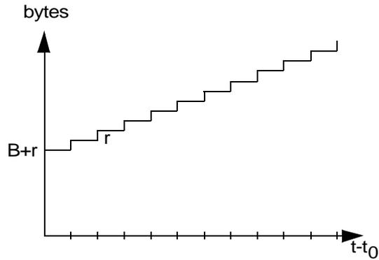
Figure 4: Token-Bucket curve in discrete time
