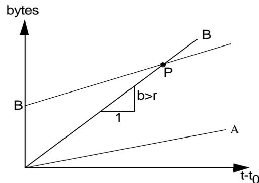
Figure 3: Flow B running out of tokens at point P
