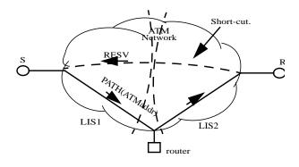
Figure 2: PATH message with source ATM address.
