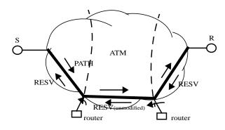
*Figure 3:* Forwarding "unmodified" RESV message upstream.
