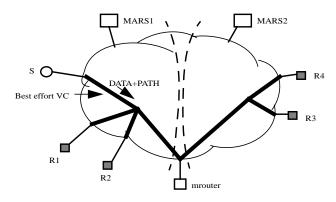
Figure 5: Multicast with multicast router (hop-by-hop).
